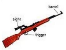
the part of a gun that the bullets are fired through
