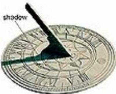
an object used in the past for telling the time. The shadow of a pointed piece of metal shows the time and moves round as the sun moves.
