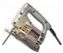
a tool for cutting out shapes in thin pieces of wood
