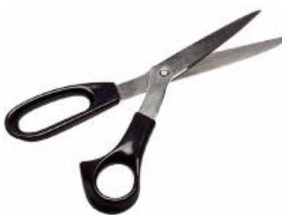
a tool for cutting paper, cloth etc, made of two sharp blades fastened together in the middle, with holes for your finger and thumb:
