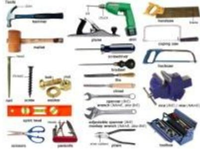
a metal tool with handles, used for holding things firmly and twisting and cutting wire
